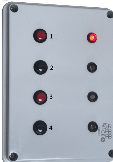
Figure 6: Example of the button box we have in the laboratory. Button 1 executes the whole program to perform General Exploration Movements + Zig Zag + Pivoting Movements. Button 2 executes only General Exploration Movements. Button 3 executes only Zig Zag Movements. Button 4 ends the program.
