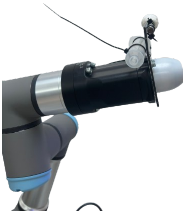
Figure 2: Transducer tool attached to the extremity of the robot.
